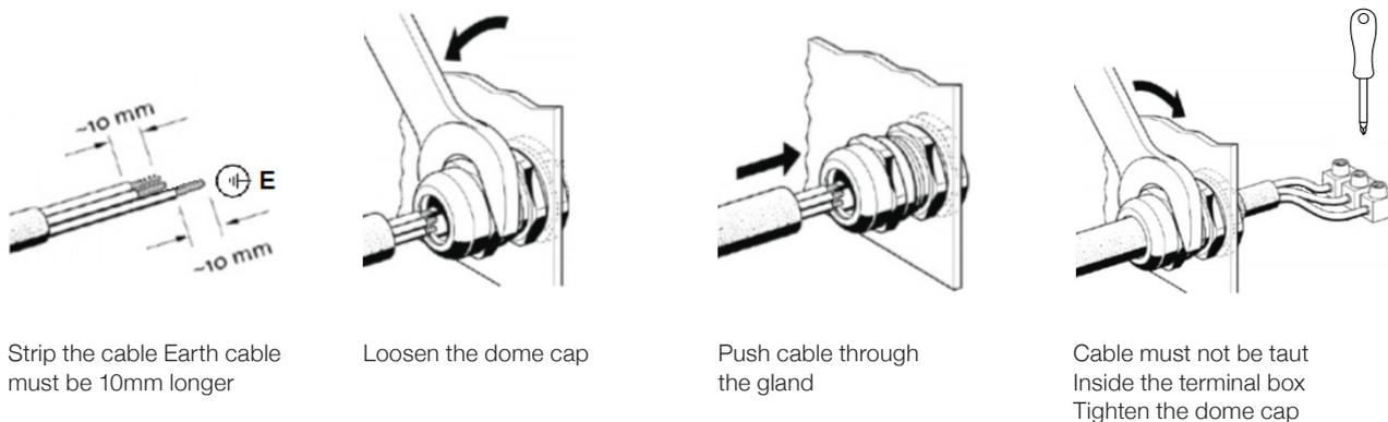
Ensure the dome cap is tightened enough that the cable is securely clamped and cannot move.
