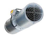
The Jetvent Axial Impulse fan range is available with either unidirectional or truly reversible airflow. Jetvent can run in either normal extract mode or once only smoke operation at up to 300°C for 2 hours which means cost savings as a single fan provides both general and smoke extract requirements.
