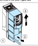
7. Frames R1...R2 and R6...R9, IP21 (UL Type 1): Install the cable boxR1...R2
