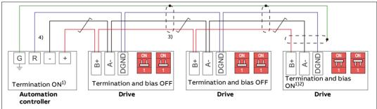
1) The devices at the ends of the fieldbus must have termination on. All other devices must have termination off.
