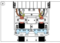
5. <u>Frame R5:</u> Install the cable box plate (a) and shroud (b). **R5**
