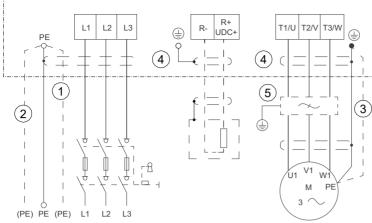
Frames R1...R3 have a built-in brake chopper. If necessary, you can connect a brake resistor to terminals Rand UDC+/R+. The brake resistor is not included in the drive delivery.
