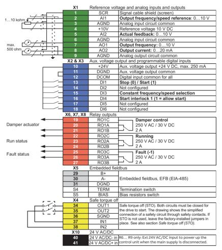
Total load capacity of the auxiliary voltage output +24V (X2:10) is 6.0 W (250 mA / 24 V DC).
