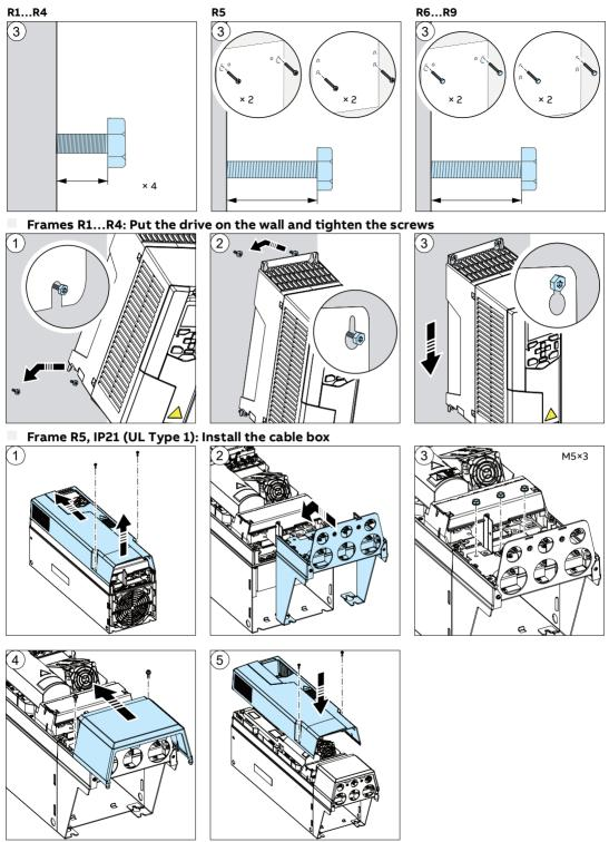
Frames R5...R9: Put the drive on the wall and tighten the screws R5 R5 R5 R6...R9
