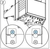
6. Remove the cover(s) R1...R4, IP21 (UL Type 1)
