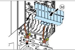
4. <u>Frames R1...R2, R4, R6...R9</u>: Install the grounding shelf. In frames R6...R9, this is the grounding shelf for the control cables.
