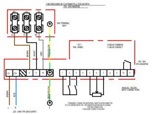
All wiring and control equipment must comply to the latest IEE regulations, in particular part 552-01-02/03. MK-152-600 lssue B: 29.04.2015
