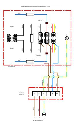
All wiring and control equipment must comply to the latest IEE regulations, in particular part 552-01-02/03. MK-152-510 Issue E: 16.08.2018 Check the individual product accessories table for fan controller compatibility.
