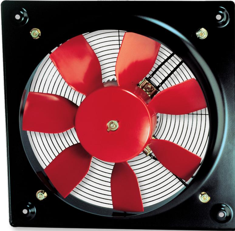
Range of low profile plate mounted axial fans fitted with plastic impellers with fiberglass, single phase motor (HCFB) or three phase motor (HCFT), IP65 (1), Class F insulation (2), equipped with thermal protection (3).
