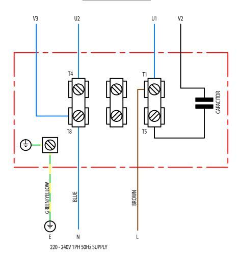
All wiring and control equipment must comply to the latest IEE regulations, in particular part 552-01-02/03. MK-152-521 Issue B: 10.09.2018
