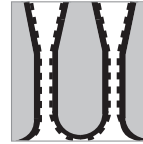
RT..QS Series Splitters with infill wrapped in impermeable film
