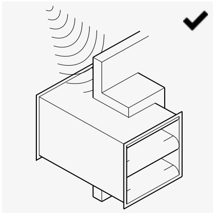
Figure 23: Acoustic sealing of silencers to achieve low noise levels
