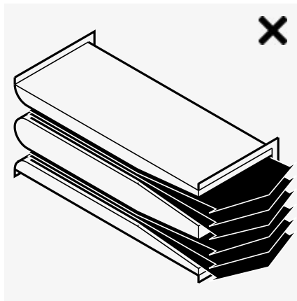
Figure 29: Airflow generated noise from silencers
