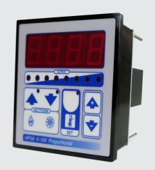
The POLA HP58 is a 0-10v thermostat or humidity controller with a single set point, programmable to monitor and control by either temperature or humidity via 2 outputs: 1x 0 to 10 Volt and 1x 3A 230Volt relay.
