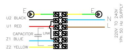
Anti—clockwise rotation (looking in the airflow direction)
