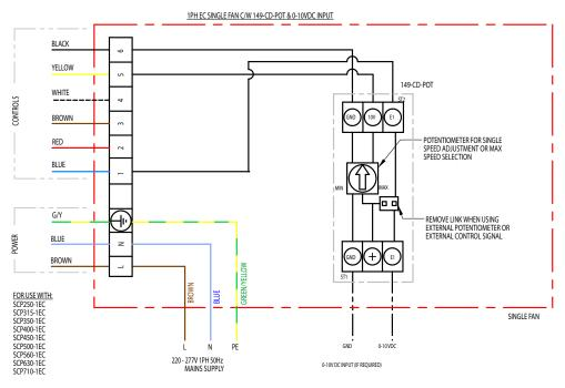
All wiring and control equipment must comply to the latest IEE regulations, in particular part BS 7671:2018+A2:2022, Regulations 552.1.2 and 552.1.3.
