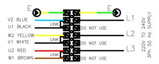
To reverse the motor rotation interchange any 2 supply phases(wires do not have markings)
