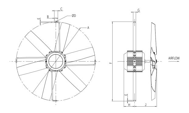
630mm unit will fit any 630-650mm tube or chimney. 710mm unit will fit any 710-730mm tube or chimney. 800mm unit will fit any 817-840mm tube or chimney.
