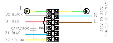
Anti-clockwise rotation (looking in the airflow direction)
